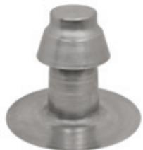
Recommended for all types of roofing systems. Install one vent per 200 sq. ft. of roof area.
